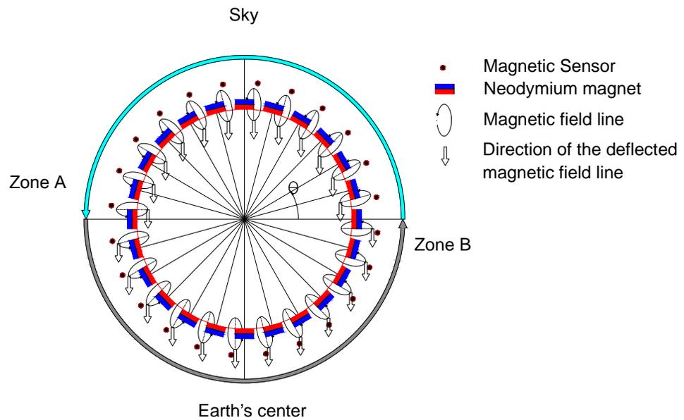
**Fig. 9. The conceptual diagram of the deflected magnetic field lines during the 360 degree of vertical rotation of the table, which are obtained from analyzing the changes in the measured magnetic flux density.**
