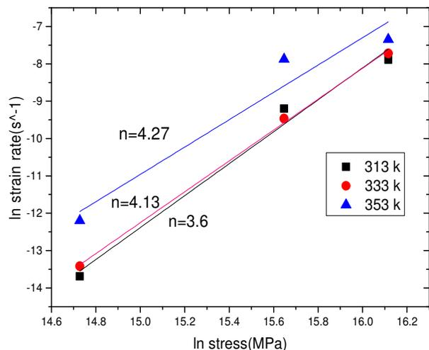
Figure 2. The relationship between  $\ln \sigma$  and  $\ln \dot{\epsilon}_s$  (sec-1) for alloys at different temperature.
