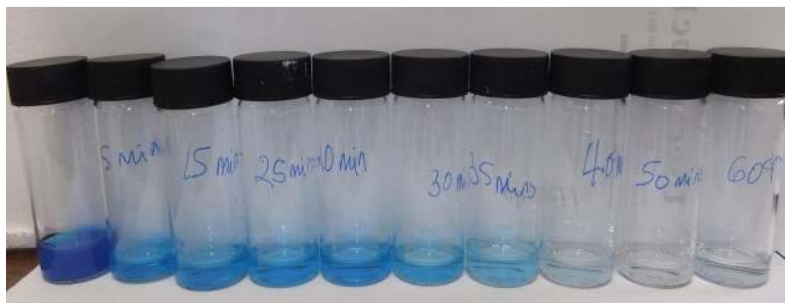
Figure 8: picture of showing the colours of CuPc dye absorbed for 0 to 60 minutes
