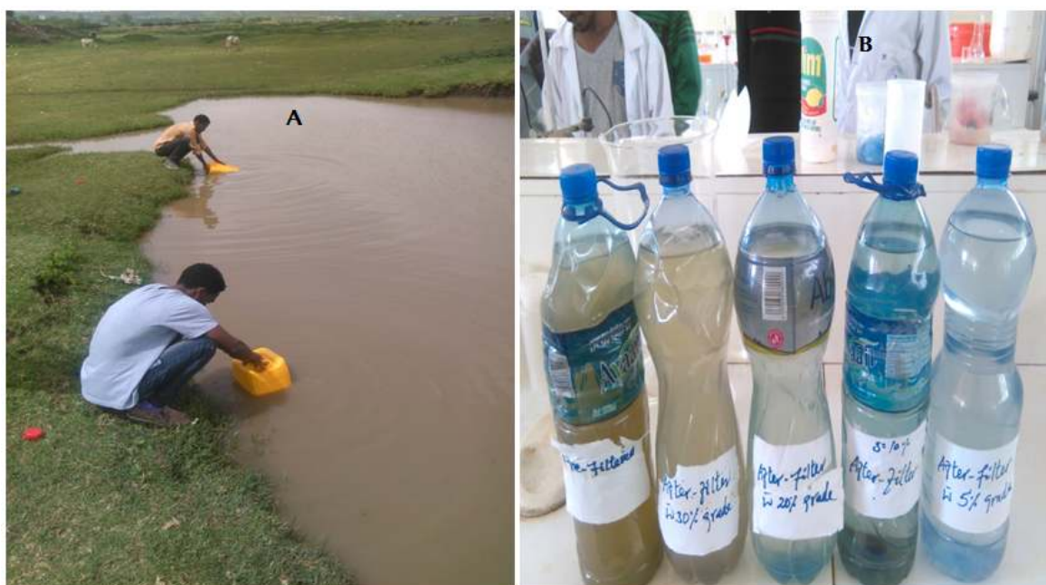
154 Figure 3: (A) sampling site (B) water samples filtered with different slopes of the sand 155 filter
