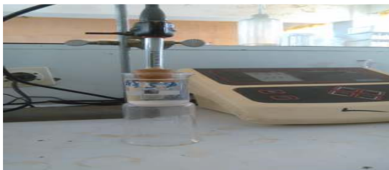
204 Figure 6: Measurement of electrical conductivity
