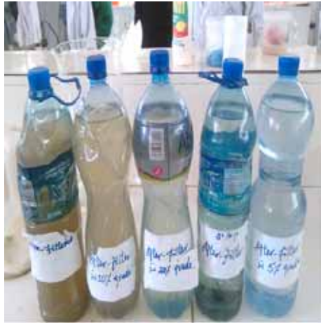
147 Figure 3: Water samples filtered with different slopes of the sand filter
