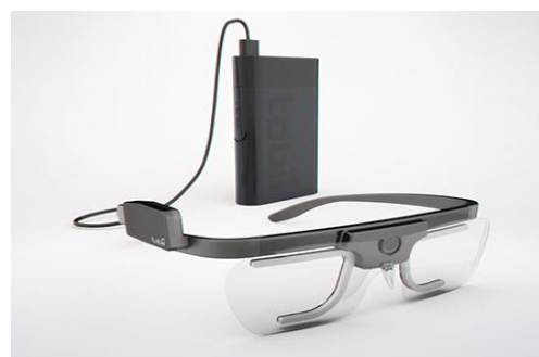
Fig. 3. SEBE equipment for French Air Force pilots: TOBII glasses 2 with external battery (the external battery may be withdrawn, limiting the autonomy to 120 minutes)
