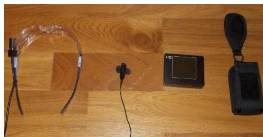
Fig. 1. SEBE equipment for NPP workers: Subcam on glasses, microphone, camcorder and bag
