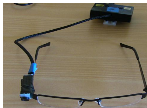
Fig. 2. SEBE equipment for Norwegian Policemen: Subcam on glasses with integrated microphone and camcorder
