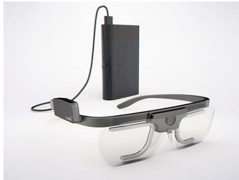
Fig. 3. SEBE equipment for French Air Force pilots: TOBII glasses 2 with external battery (the external battery may be withdrawn, limiting the autonomy to 120 minutes).
