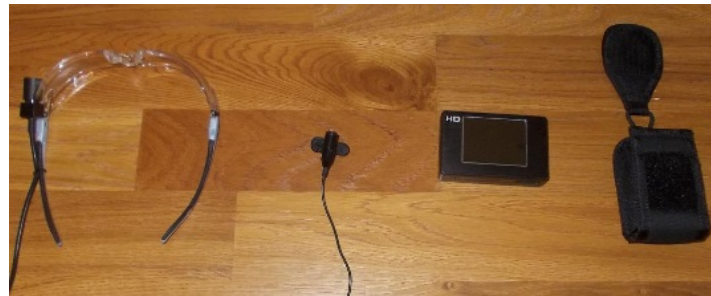
185 Fig. 1. SEBE equipment for NPP workers: subcam on glasses, microphone, camcorder and 186 bag. 187
