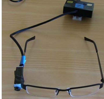
Fig. 2. SEBE equipment for Norwegian Policemen: subcam on glasses with integrated microphone and camcorder.
