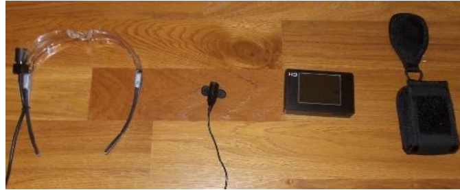
145 146 Fig. 1. SEBE equipment for NPP workers: subcam on glasses, microphone, camcorder and bag. 147
