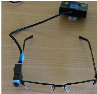
158 159 Fig. 2. SEBE equipment for Norwegian Policemen: subcam on glasses with integrated microphone 160 and camcorder. 161
